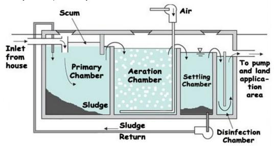
The enhanced wastewater near the top of this compartment finally passes to the irrigation tank where it is disinfected, usually by chlorine and then pumped to the designated irrigation area (land application area).
