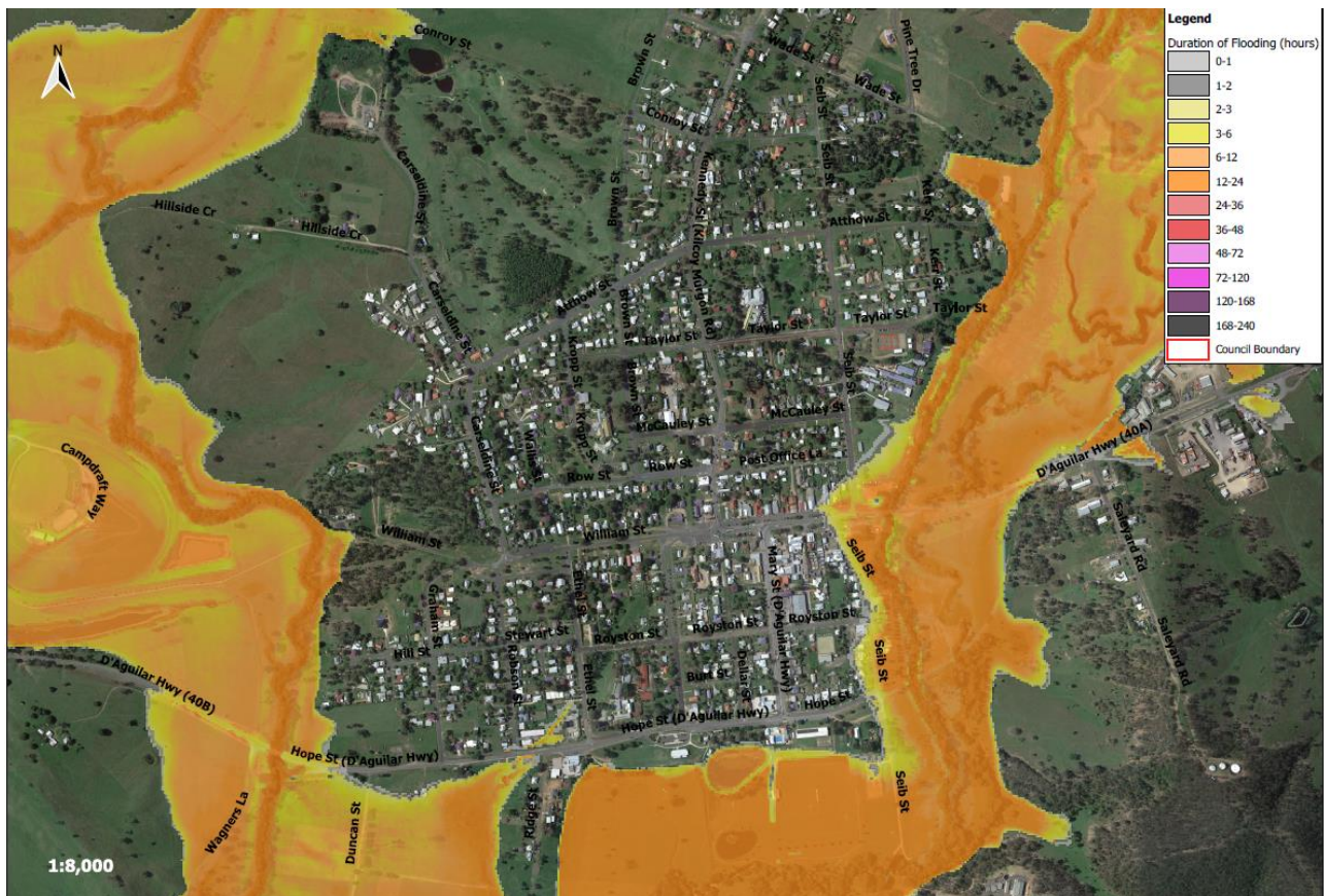
FIGURE 3-9 KILCOY TOWNSHIP DURATION OF INUNDATION 1 IN 100 AEP
