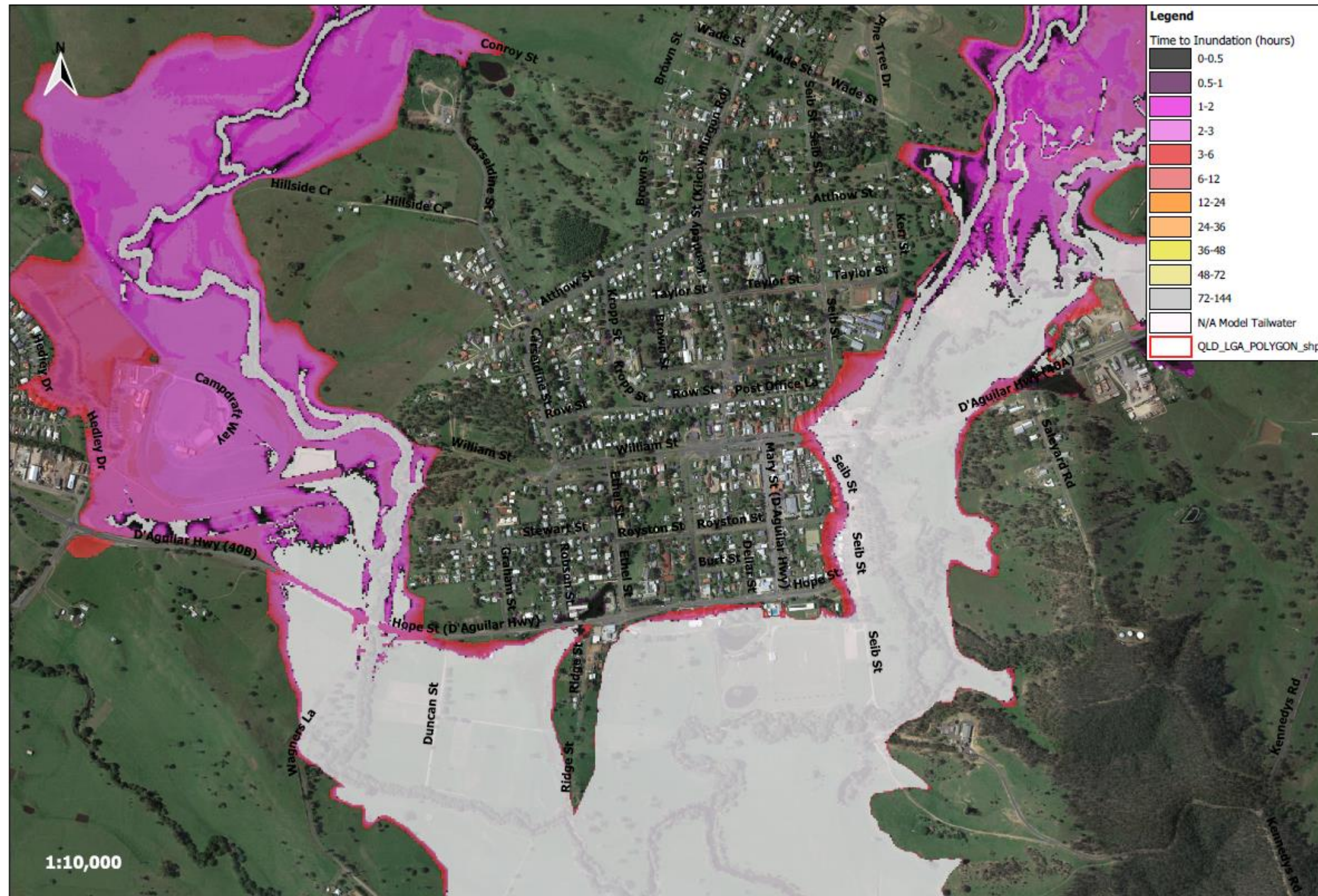
FIGURE 3-3 TIME TO INUNDATION (1 IN 2000 AEP) GROUND SURFACE
