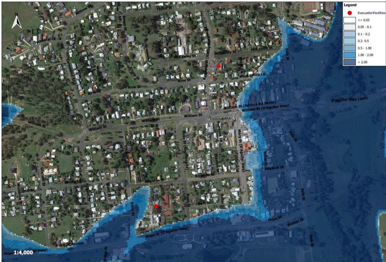
FIGURE 9-4 KILCOY EVACUATION CENTRES PMF FLOOD DEPTH
