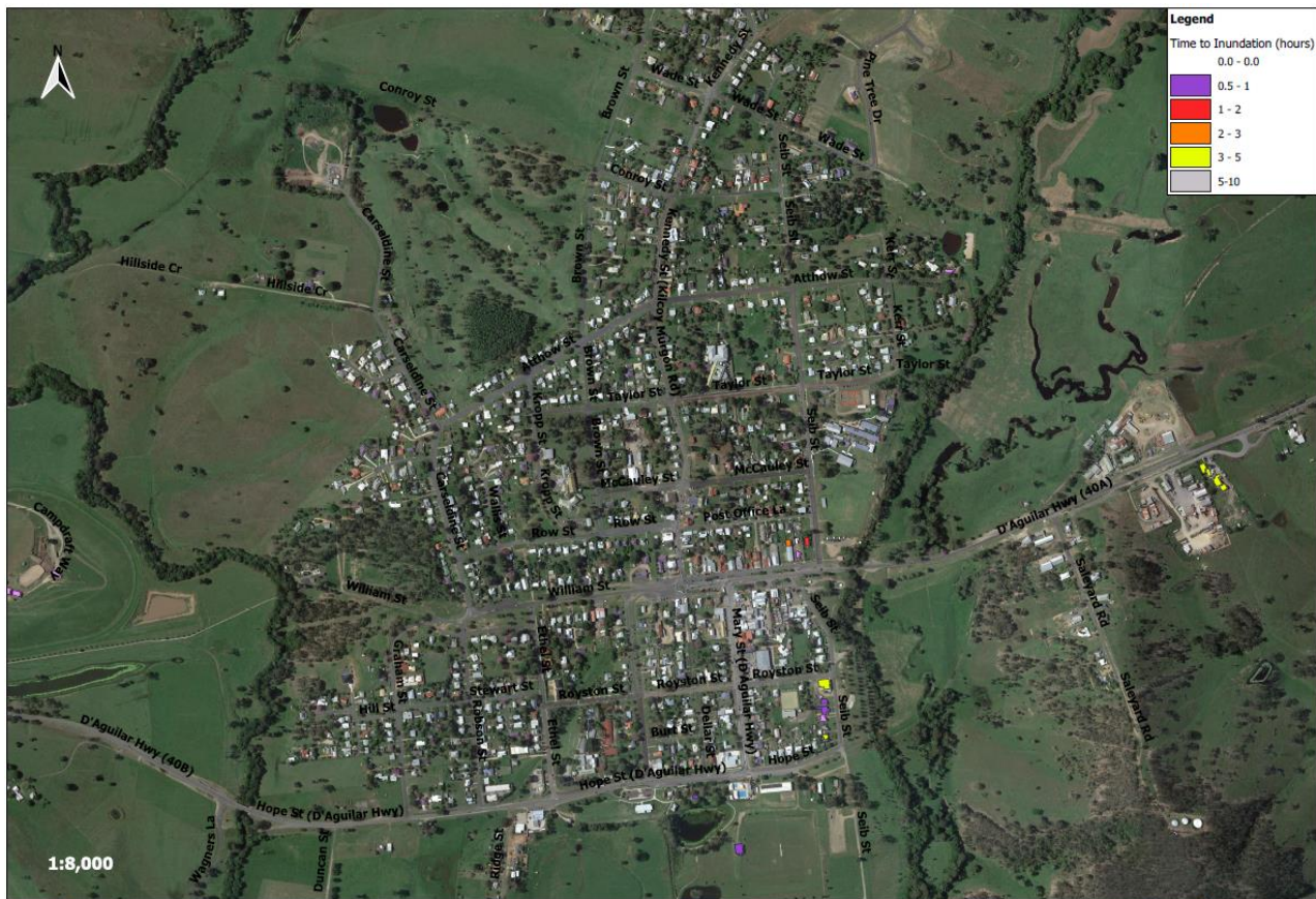
FIGURE 3-7 BUILDINGS – TIME TO INUNDATION
