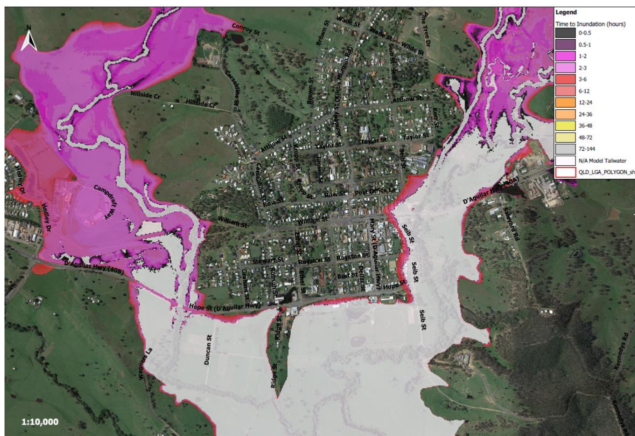
FIGURE 3-5 KILCOY TOWNSHIP CATCHMENT TIME TO INUNDATION (1 IN 2000 AEP)
