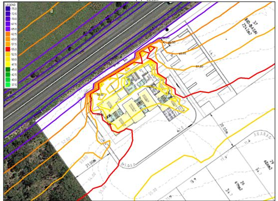
Table B3: Receiver point calculations, 2033. Levels are in dB(A) L<sub>10,hr</sub> façade-affected
