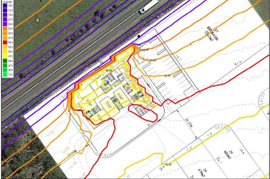
Table B5: Receiver point calculations, 2032, 3.5m fence scenario. Levels are in dB(A)  $L_{10,18hr}$  façade-affected
