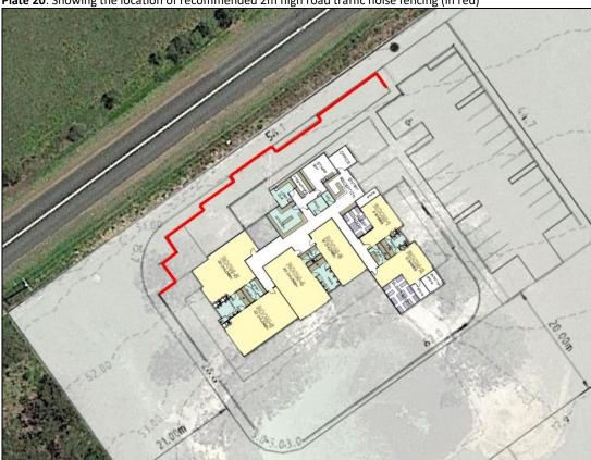
Plate 20: Showing the location of recommended 2m high road traffic noise fencing (in red)
