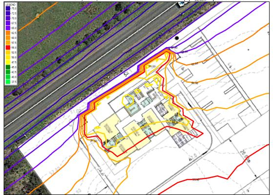
Table B5: Receiver point calculations, 2033, 3.5m fence scenario. Levels are in dB(A) L<sub>10,18hr</sub> façade-affected
