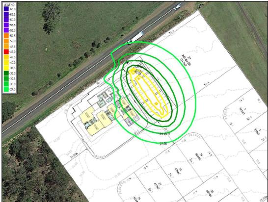
Table C3: Receiver point calculations, car door 'slam'. Levels are in dB(A) L<sub>max</sub>
