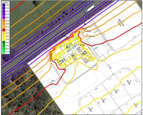
Table B3: Receiver point calculations, 2032. Levels are in dB(A) L<sub>10,18hr</sub> façade-affected
