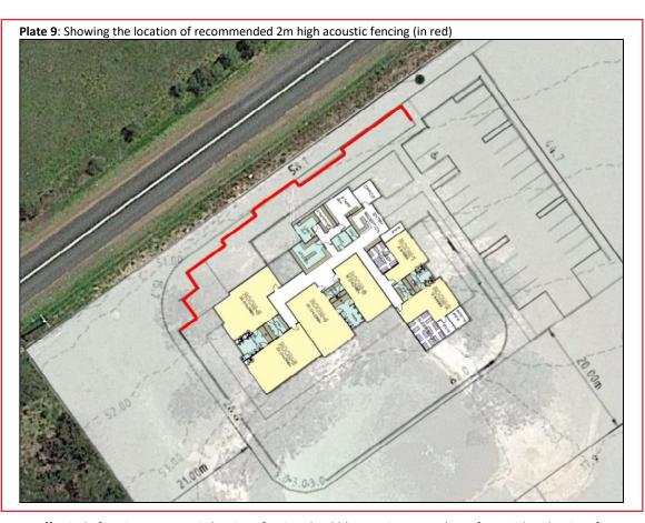
Construct a 2m noise barrier in accordance with condition 10 (a)-(b) of the referral agency response.
