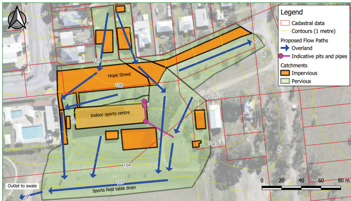
Figure 7: Existing Site Catchments and Flow Paths with Alternate Distribution
