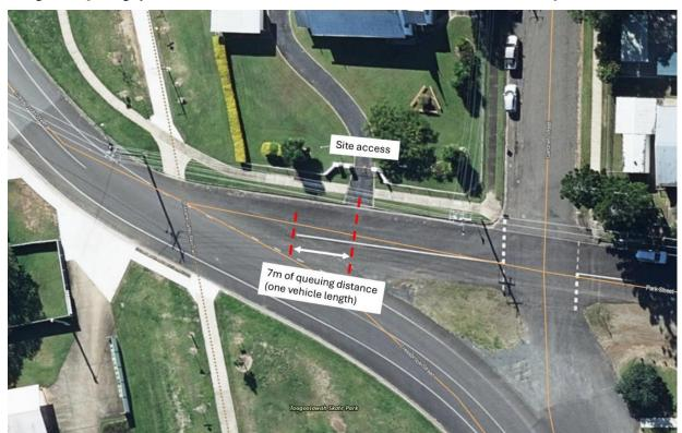
Figure 4: Queuing space between site access and Cressbrook Street intersection (Source: Queensland Globe)
