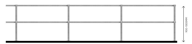
Fence Type D: Typical Elevation
